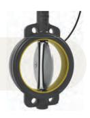
After the disc rotates, the air is supplied to inflate the seat. The operation method enable no friction occurs between the seat and the disc, damage and wear of the seat are minimized, and the valve has the longer life cycle.
